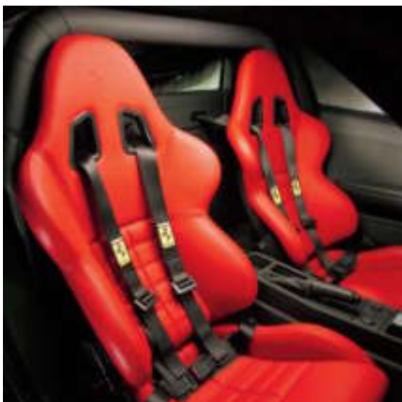
Sedili racing in fibra di carbonio con cuciture a quattro punti e roll-bar stradale Carbon-fibre racing seats with four-point harness and road roll-bar
